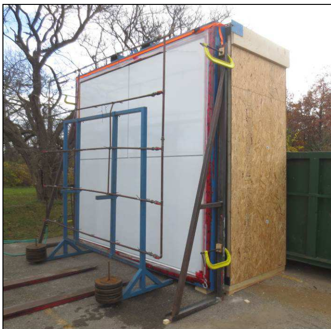
Figure C2 - Spray rack Set up for water penetration
